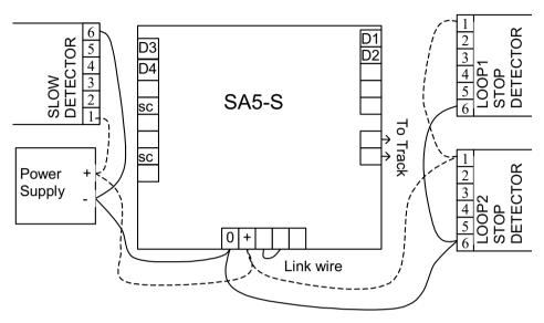
track set the direction the train moves. Reverse these if the train is travelling in the wrong direction. Adjust the maximum speed to the desired setting.
