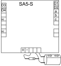
the end of the first passing loop. The train will stop and the red and green lights flash alternatively then the train will accelerate away. On the second lap, D3 will again slow the train but D2 will halt it, as the points would now have set for the second loop. Check the IRDOT-1s are wired correctly by placing your hand over the detectors in the same order. Note that the detectors must operate in the correct sequence. A train must operate D3 before it can be stopped by D1 or D2.
