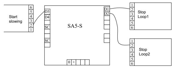
terminal 2 of the loop 1 IRDOT to D1. Wire from terminal 2 of the loop 2 IRDOT to terminal D2.
